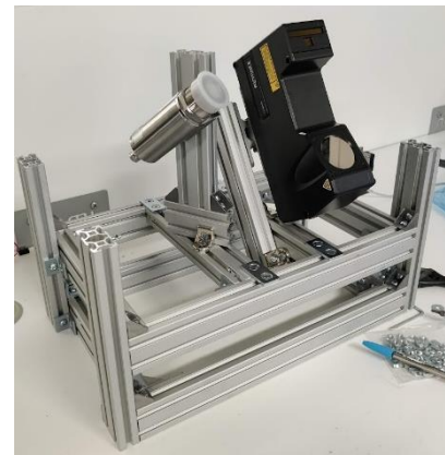
Figure 3. Photograph of the profilometer and thermal camera on the support.
